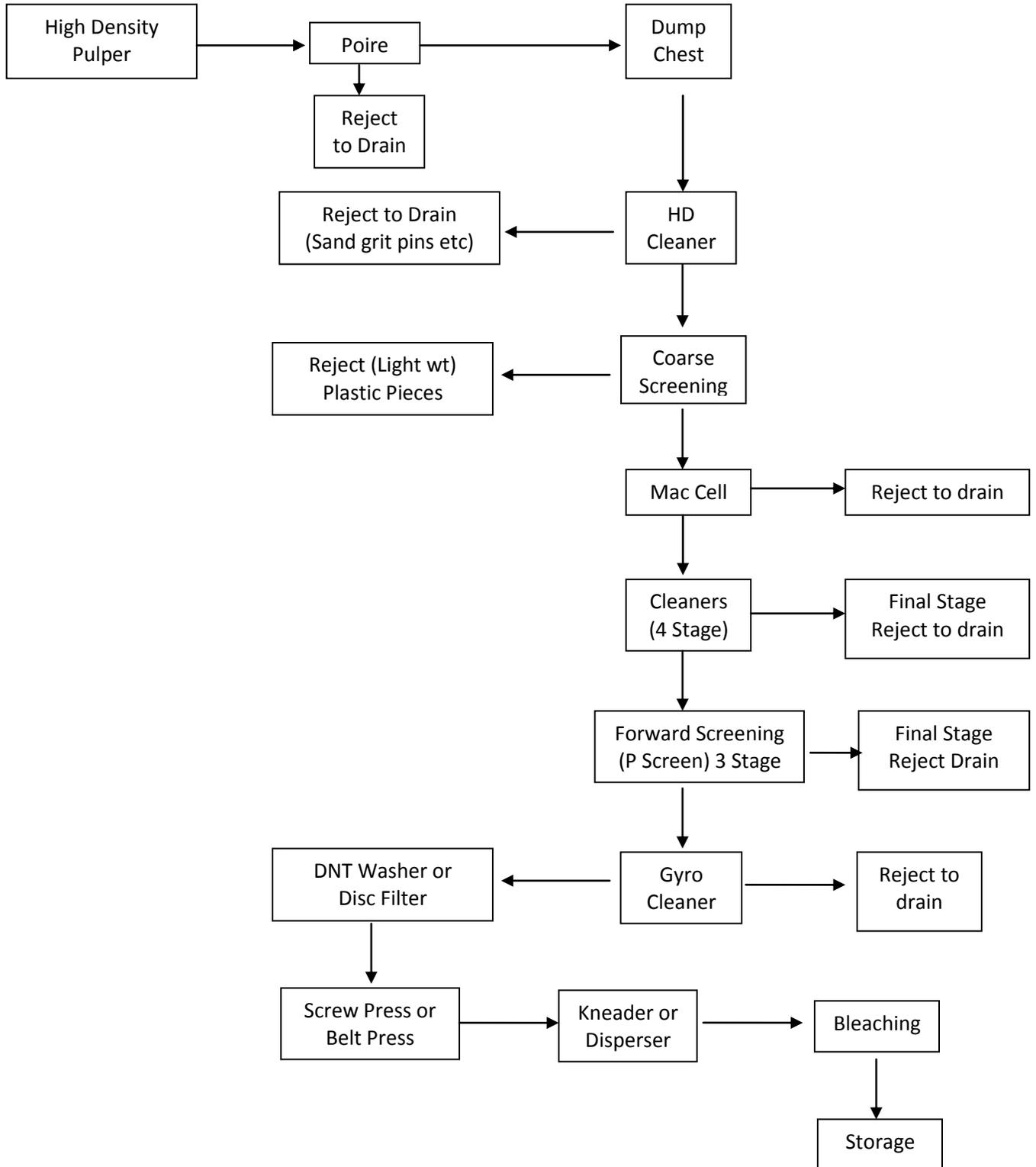
In the above system the filtrate obtained from DNT washer or disc filter, screw press or belt press and kneader or disperser unit are clarified in a Poseidon or DAF unit. This clarified back water is used in dilution at different stages in the process. The rejects from Mac cell and reject from Poseidon or DAF unit is processed through decanters or belt presses as a disposable sludge.
