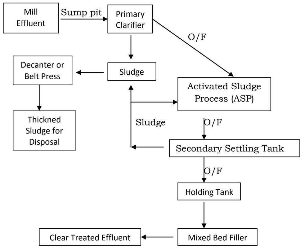
In case of higher volumes, one need to install secondary clarifier after the secondary treatment. This type of elaborate arrangement may not be practicable in many cases due to financial, operational and other reasons. The above system ensures the final effluents are within the disposal norms and can be utilized for reuse, for land disposal for irrigation or disposal in to CETP line or into the receiving stream.
